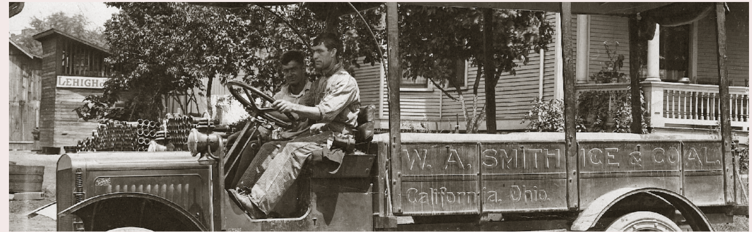
William A. Smith at the wheel of his Ice & Coal Company delivery truck in about 1918. The truck had a chain drive, solid tires and side curtains.
